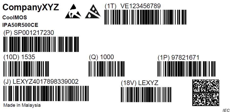
Figure 1 – Label with a linear bar code, Data Matrix symbol and human-readable information
